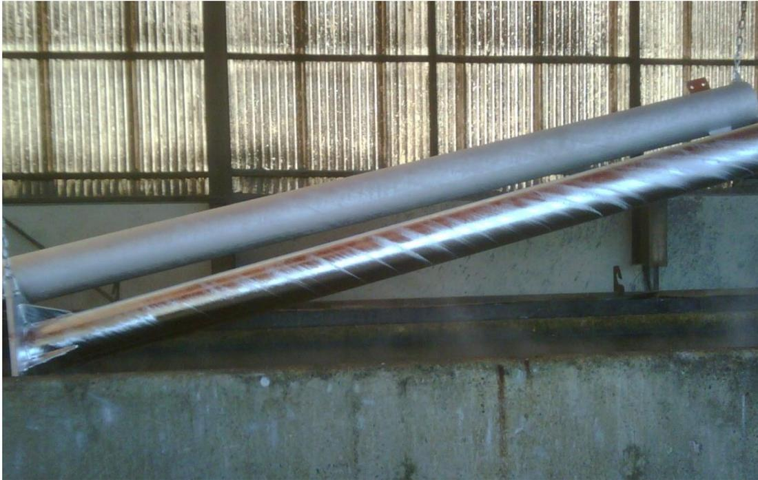
**Figure 2:** Two posts with different steel compositions after being galvanized at the same time. The top post is typical of steel from Categories C & D while the bottom appearance is typical of steel from Categories X & A. Both products comply with AS/NZS 4680.
