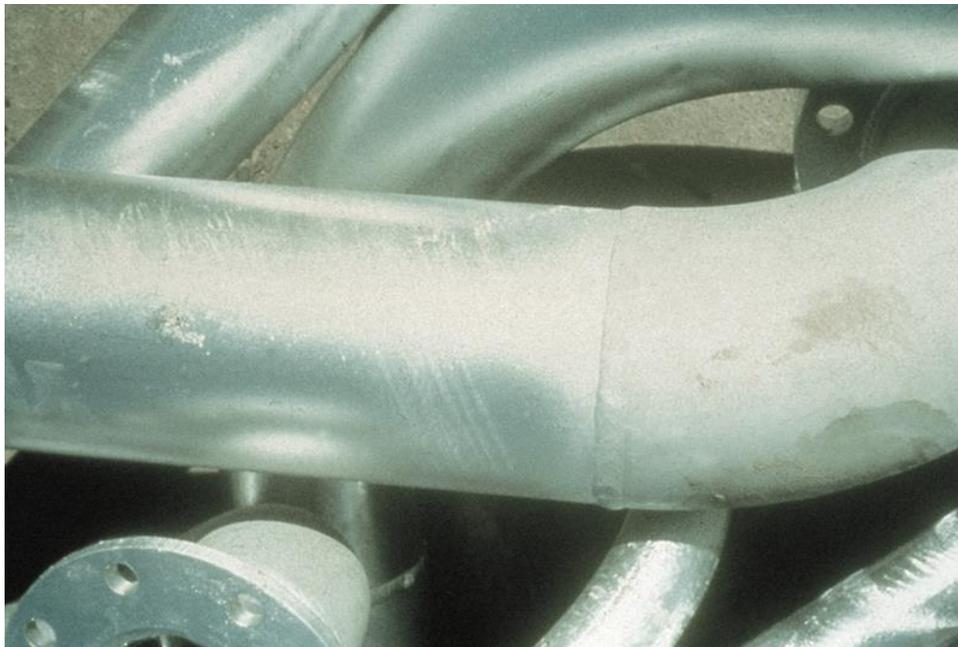
**Figure 7:** The shiny surface (to the left) is typical of Category X, A & B, while the duller coating (to the right) is typical of Category C & D. Over time, the both coatings will weather and tend towards a similar dull grey colour. This product meets the requirements of AS/NZS 4680.
